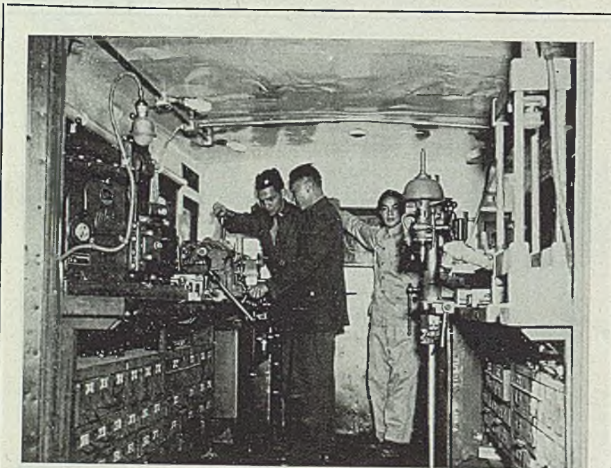
AID TO CHINESE: Latest United States Army contribution to the Chinese offensive against the Japanese on the Salween front is a number of General Motors 2½-ton ordnance machine shop mobile trucks. Shown in the photo above is Maj. Harold H. Morse, Kansas City, Kans., showing Maj. Gen. Siu Ho, commanding general of Chinese ordnance, equipment in the shop truck, which includes a bench shaper, lathe, drill press, bench grinder, portable electric drills and a 5-kw generator set. Signal Corps photo
