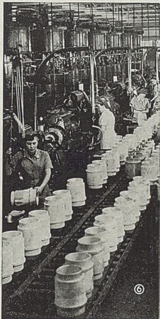
floor space; 9 machines; $33,600 over cost of standard machines and fixtures; 2 handling operations; 28 men and 214 production hours per 3-shift day
