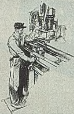
Making sure LST shaft is true.
