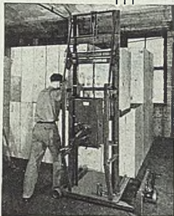
Hand Model REVOLVATOR with revolvable base piling cases containing delicate x-ray equipment.
