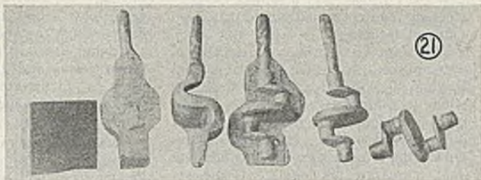
Fig. 21—Illustration of various steps in the forging of a small crankshaft
