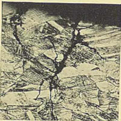
Fig. 1. Photomicrograph of yellow brass tubing showing transcrystalline cracks starting at surface.
