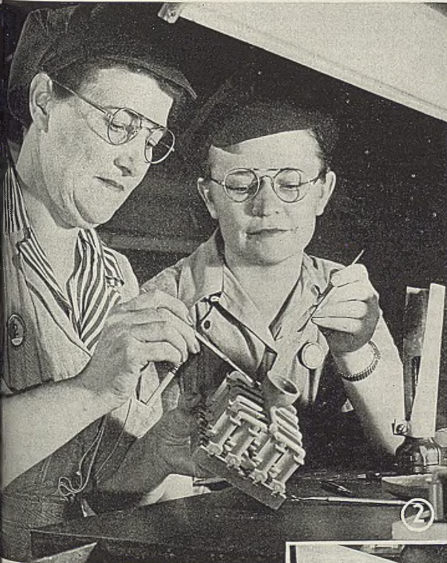
Fig. 4—Any defective bucket patterns are cut from the riser and good ones substituted. Work is done on a match plate to assure proper dimensions and alignment of assembly
