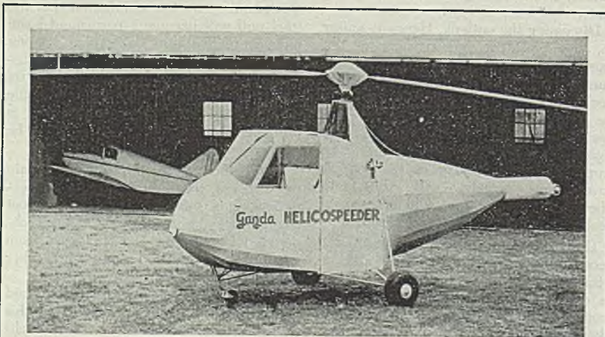
JET-PROPELLED HELICOPTER: The usual auxiliary rotor fixed at the tail of orthodox helicopters is omitted in this jet-propelled and jet-steered "Helicospeeder" invented by Antoine Gazda. More speed, weight-carrying capacity, stability and controllability are claimed for the craft. NEA photo
