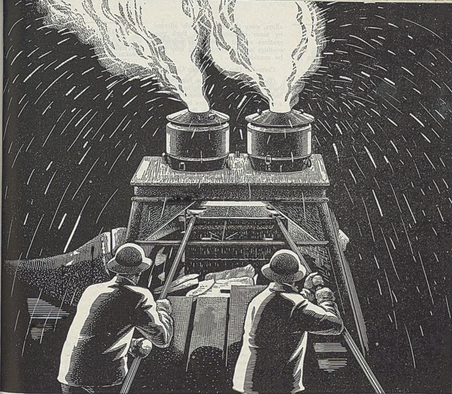
Pouring a double Themit weld in fabricating a ship stern frame.
