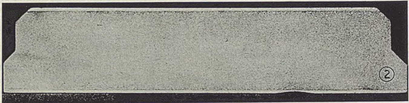
Fig. 3—Cross section of product which has only one surface of cupronickel
