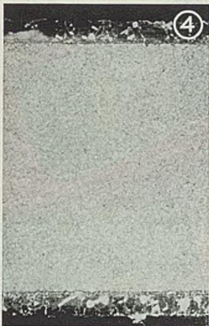
Fig. 4—Cross section of laminated plate at high magnification showing bonding and grain structure
