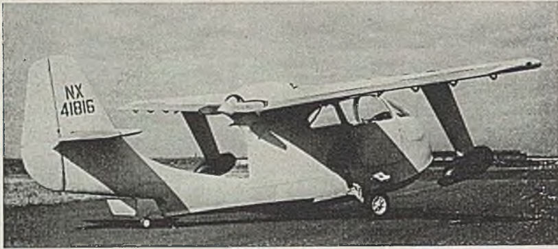
THUNDERBOLT AMPHIBIAN: Although P-47 Thunderbolts still are coming off the lines at full speed at the plants of the Republic Aviation Corp., engineering thought is being given to postwar flying. Above is shown a tentatively designed Thunderbolt amphibian just before taking off on a test flight. At its present stage of development, the craft is an all-metal high-wing ship, powered by a 175-horsepower engine, will accommodate four passengers and is intended to sell for less than $4000
