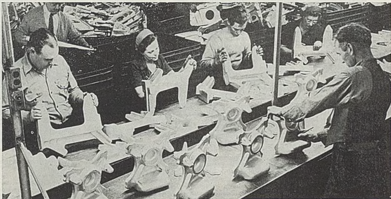
Indicative of the variety and grotesque shape of typical aluminum forgings used in combat airframes is this view of one of the inspection benches at the Dodge aluminum forge plant in Detroit. This plant has produced literally hundreds of types of forgings for over 20 different fighter planes and bombers and was built specifically for this type of production. Steam hammers range up to 20,000-pound size. Most forgings are of 14ST alloy
