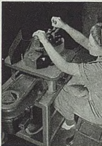
Above: An outstanding example of the adaptation of a standard Delta-Milwaukee Shaper to an especially tough job — shaping magneto timing cams to exact tolerance of .0005". Thus a $35.00 machine does a job which could be done no better by the grinding machine ordinarily used for this work and costing about $1500.00. The addition of a special fixture was necessary in either case, so the fixture cost remained the same.
