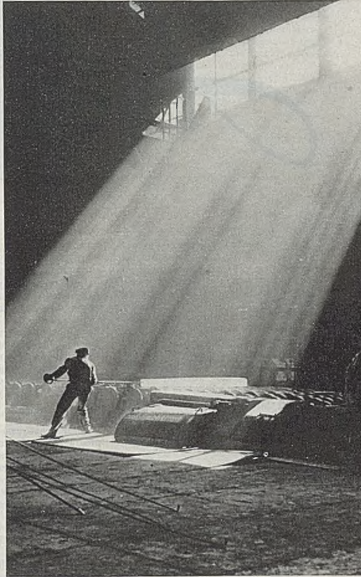
During the rolling process the constantly thinning slab goes from one set of rolls to another. Here in an Alabama mill a workman is turning a slab so that it will enter the next pass broadside. United States Steel Corp.
