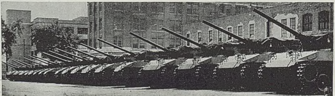
"Hellcat" of the ground forces is the 19-ton, 55-mile-an-hour tank destroyer built by Buick and used extensively in the invasion of Europe
