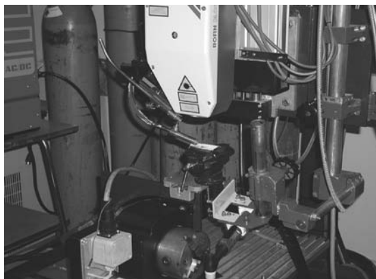
Fig. 1. HPDL laser Rofin DI 020 used for remelting and alloying of the hot work tool steel samples
