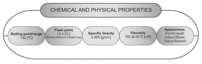
Fig. 5. Chemical and physical properties of medical silicone MDX4-4159 manufactured by COW CORNING
