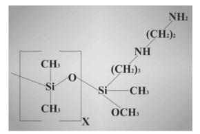
Fig. 4. The diagram of the Dow Corning silicone structure MDX4-4159, 50% Medical Grade Dispersion
