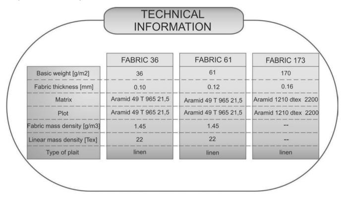
Fig. 2. Technical information about aramid fabric manufactured by Havel Composites PL. SP. Z O.O
