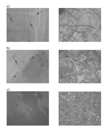
Fig. 11. Surface of samples made based on aramid fabric with basic weight a) 36 g/m<sup>2</sup>, b) 61 g/m<sup>2</sup>, c) 173 g/m<sup>2</sup>(the vacuum chamber); 40x. Left side – top surface of samples, right side – contact with base bottom surface
