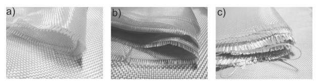
Fig. 3. Aramid fabric with basic weight a) 36g/m<sup>2</sup>; b) 61 g/m<sup>2</sup>; c) 173g/m<sup>2</sup>
