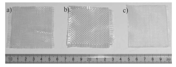
Fig. 8. The survey of prepared samples taken from aramid fabric with basic weight a)  $36g/m^2$ ; b)  $61 g/m^2$ ; c)  $173g/m^2$
