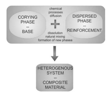
Fig. 1. Composite materials definition - graphic diagram [20]
