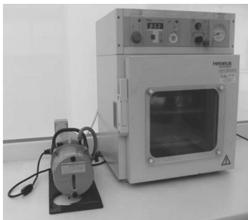
Fig. 8. The heat vacuum chamber: Heraeus Instruments - Vacuotherm (Kelvtron:t)
