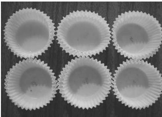
Fig. 5. The samples of pure silicone before hardening
