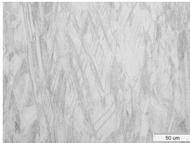
Fig. 7. Single – phase structure of bronze CuSn7 with the shear bands; tensile temp. 250°C, break–off zone of the sample; 500x
