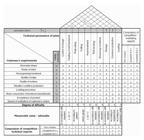
Fig. 3. House of Quality for hot rolling steel
