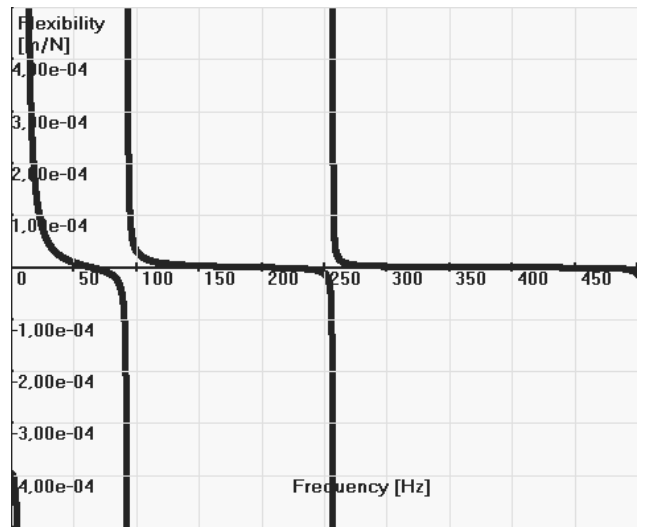
Fig. 7. The dynamical flexibility (18) of stationary free-free beam
