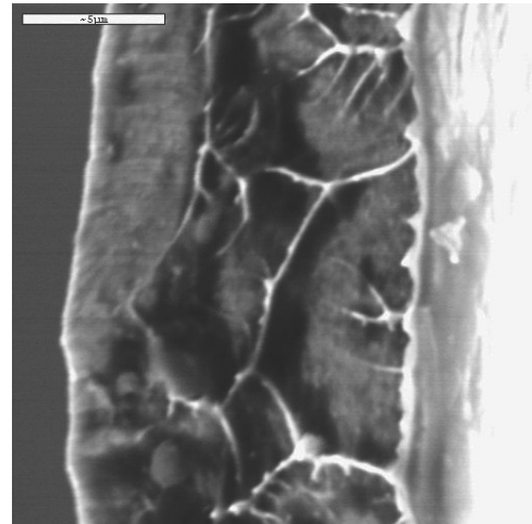
Fig. 13. SEM image of the ductile fracture with vein pattern morphology of amorphous Co_{68}Fe_4Mo_1Si_{13.5}B_{13.5} ribbon in as-quenched state
