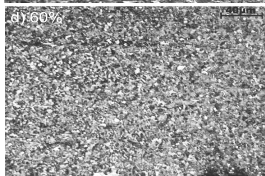
Fig. 8. Stress-strain curves of the 27Mn-4Si-2Al steel – (a), and austenitic structures of the specimens solution heat-treated from 850°C after deformation 20% (b), 40% (c) and 60% (d)
