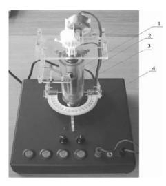
Fig. 1. Apparatus for MR effect measurement. 1 - shaft (drive) and inner cylinder, 2 - outer cylinder, 3 - coil, 4 - neddle and angular displacement scale
