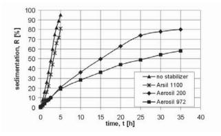
Fig. 4. Sedimentation ratio vs time for MR fluid containing different stabilizer (OKS 600, 7.3 mPa·s, CI 20%)
