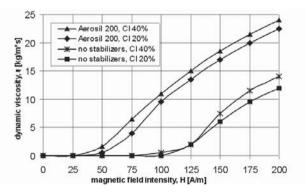
Fig. 2. Dependence of the MR fluid (OKS 1050, 150 mPa·s) dynamic viscosity on the magnetic field intensity
