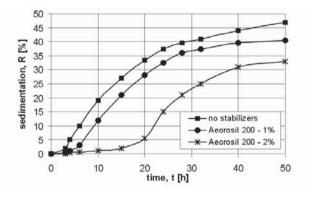
Fig. 6. Sedimentation ratio vs time for MR fluid with different stabilizer content (OKS 1050, 500 mPa·s, CI 40%)
