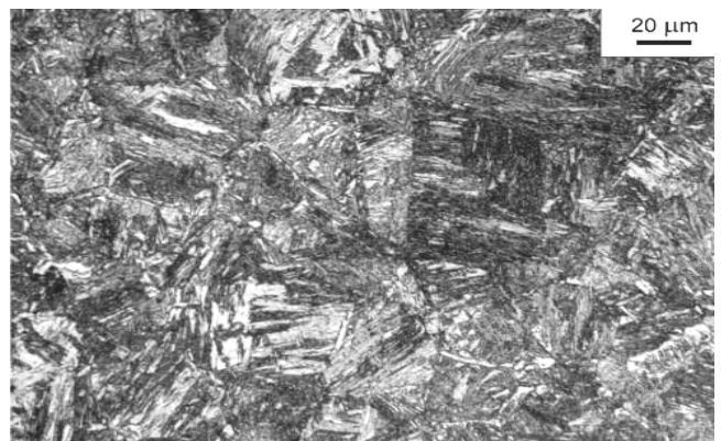
Fig. 7. Lath martensite structure containing retained austenite of the specimen water-quenched from 1200°C
