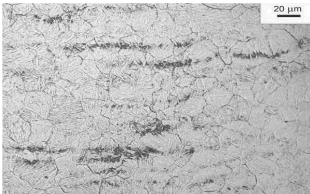
Fig. 4. Structure of primary austenite of the specimen water-quenched from a temperature of 1000°C
