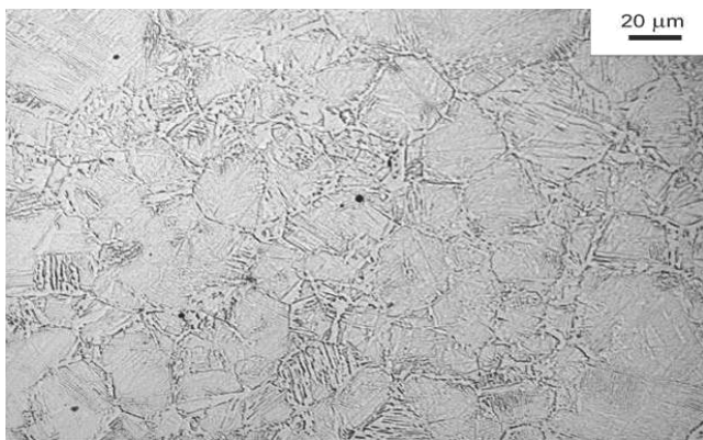
Fig. 5. Structure of primary austenite of the specimen water-quenched from a temperature of 1100°C
