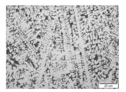
Fig. 1. Central zone of the remelting surface layer of X40CrMoV5-1 steel after alloying with NbC, power range 1.2 kW
