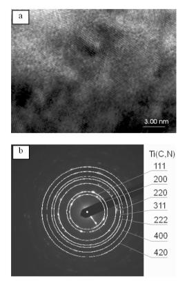
Fig. 5. a) Structure of the thin foil from the TiCN coating deposited onto the hot work tool steel X40CrMoV5-1, b) diffraction pattern from the area as in figure a) and solution of the diffraction pattern
