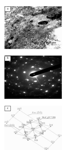
Fig. 4. Structure of the thin foil of X40CrMoV5-1 steel, after alloying NbC, power of bunch laser 1.6 kW: a) a picture in a bright area, a diffraction pattern of area as fig. a), a solution of diffraction pattern from fig. b)
