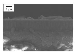
Fig. 3. Fracture of the TiAlN coating deposited onto the X40CrMoV5-1 steel substrate
