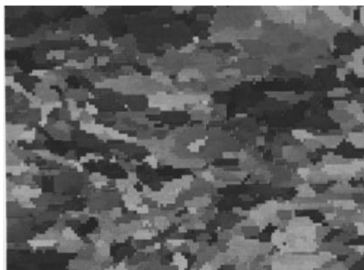
Fig. 10. Crystall oriented map, sample after 8 ECAP passes
