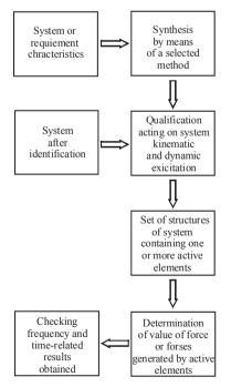
Fig. 1. Idea of synthesis of active mechanical systems
