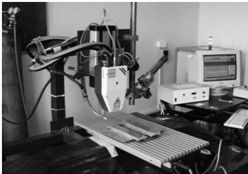
Fig. 1. HPDL laser welding test stand
