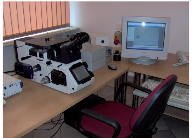
Fig. 2. The real laboratory post with the light microscope Leica MEF 4A / M placed in the Institute of Engineering Materials and Biomaterials at The Silesian University of Technology [11].
