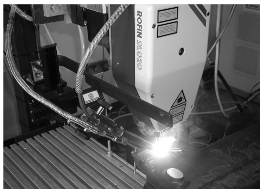
Fig. 1. Alloying process of ceramic particles of hot work tool steel using high power diode laser HPDL Rofin DL 020
