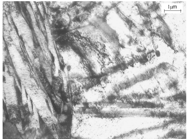
Fig. 9. A part of the martensitic island in the ferrite matrix of high dislocation density
