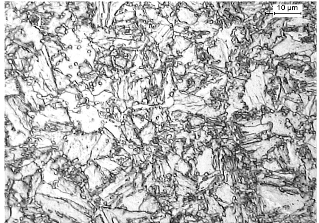
Fig. 6. Ferritic – martensitic structure of the steel twice quenched from the temperatures of 910°C and 750°C
