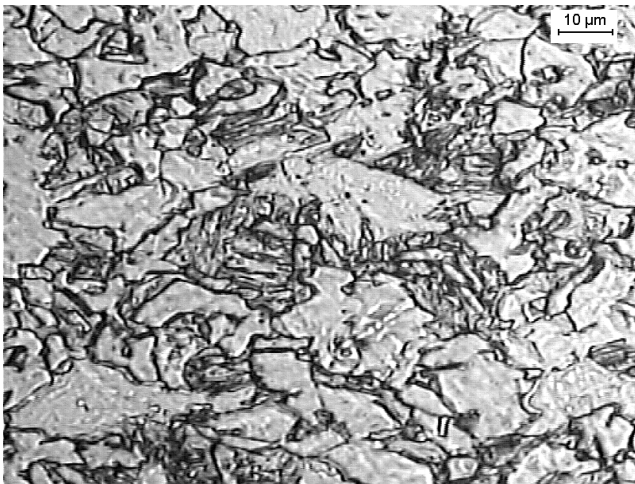
Fig. 8. Ferritic – martensitic structure of the steel quenched from a temperature of 785°C after previous air cooling for 35s from 910°C
