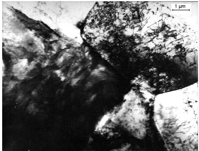
Fig. 10. Martensitic island on the boundaries of three ferrite grains of high dislocation density
