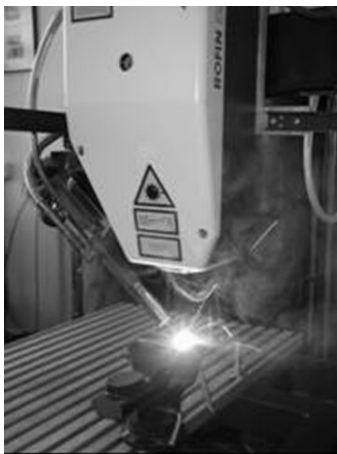
Fig. 2. Alloying process of ceramics particles of hot work tool steel using high power diode laser HPDL Rofin DL 020
