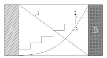
Fig. 1 Type of gradient: 1- linear; 2- stepped; 3- parabolical
