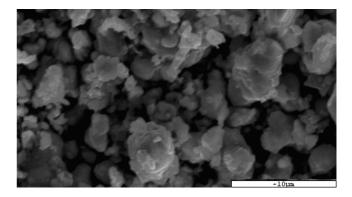
Fig. 3 Powder of (W, Ti)C with cobalt
