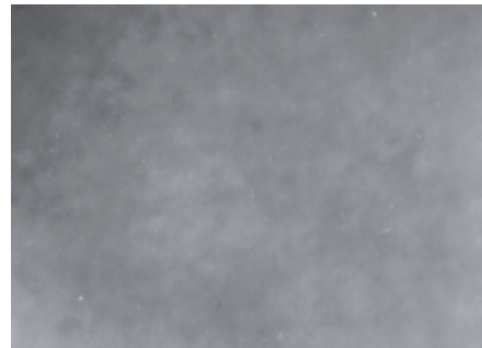
Fig. 1. Structure of Co 70,5 Fe 2,5 Mn 4 Mo 1 Si 9 B 15 amorphous alloy at quenched state, with characteristic contrast (TEM, thin foil, magnification 80 000x)
