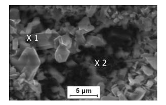
Fig. 3. Surface morphology the coating after isothermal oxidation test  $900^{\circ}C/500h$
