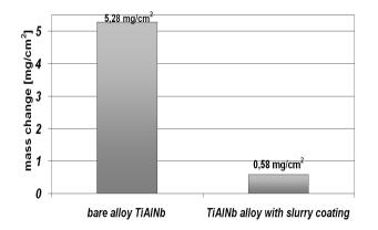
Fig. 2. Mass change in the samples after the isothermal oxidation test  $900^{\circ}C/500h$
