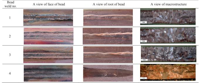
**Remarks:** welding parameters: welding speed – 100 [mm/min], laser beam power 2,2 [kW], Beads no. 1 and 3 were welded on austenitic backup, bead no. 4 was welded on argon backup
