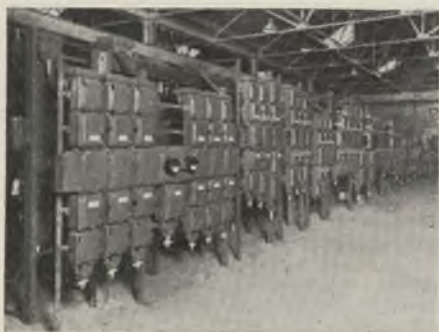
Part of consignment of medium voltage distribution switchgear supplied to the U.S.S.R.
