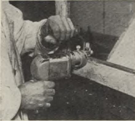
The Bilton-Scratchley window putty router being operated
