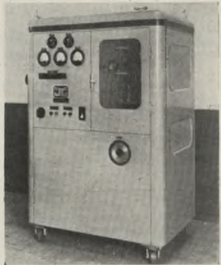
Fig. 2.—Typical equipment for pre-heating moulding pre-forms
