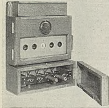
Indicator panel of new fire alarm system, showing the plug and jack arrangement for isolating alarm bells and operating indicator lamp
