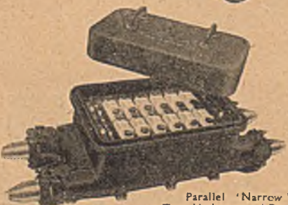
Parallel 'Narrow' Type Underground Disconnecting Box with Bolt on Wiping Glands. The fuses are provided with Porcelain Carriers which can be fitted instead of the Bakelite Lifting Bars supplied as standard.
