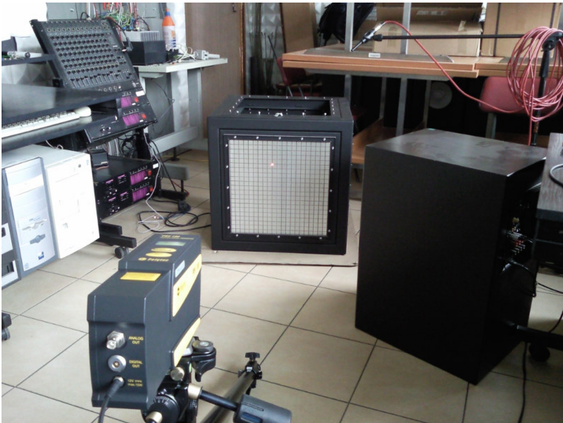
Figure 4.4: The laboratory setup with the laser vibrometer and the rigid casing used to measure modeshapes of the casing walls.
