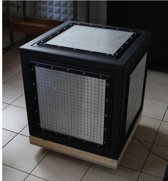
Figure 2.2: A photograph of the rigid active casing (Wrona and Pawelczyk, 2014b).
