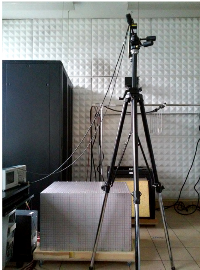
Figure 4.13: The laboratory setup with the laser vibrometer and the light-weight casing to measure modeshapes of the structure.
