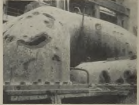
The l.p. cylinder of one of the Fulham sets
