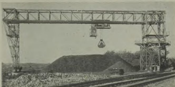
The coal-dumping ground is served by a travelling (swivelling) telfer crane which operates over a semi-circular area
