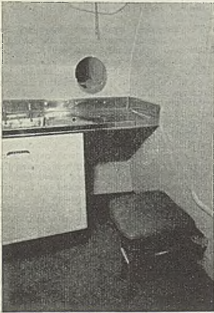
One of the toilets with an illuminated mirror on the right. The cupboard houses the water storage heater
