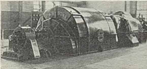
16 000 kW 3 000 r.p.m. Parsons turbo-alternator in an industrial plant in Canada
