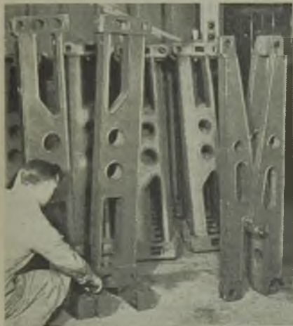
Fabricated posts for the Bailey pontoon bridge and (right) converting 2-pdr. naval pom-pom mountings from hand to power operation at the Ferguson, Pailin works
