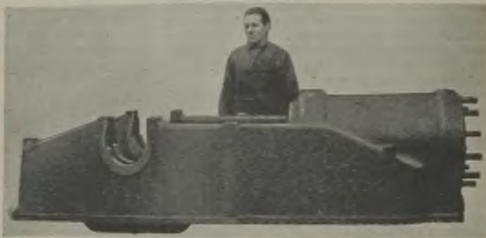
Damaged bedplate of a 80-HP horizontal oil engine which was expeditiously restored to service
