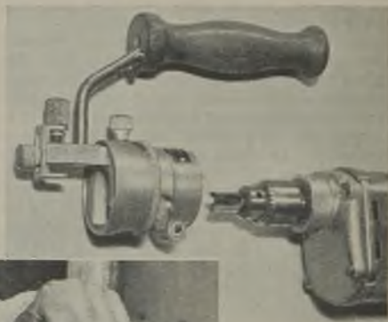
Bilton-Scratchley putty remover showing its use together with a lightweight hand drill
