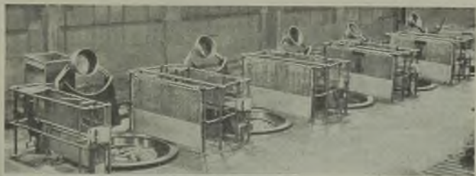
Above: Oil carried on the swarf is thrown off while in the "whizzing" baskets of the centrifugal machines
