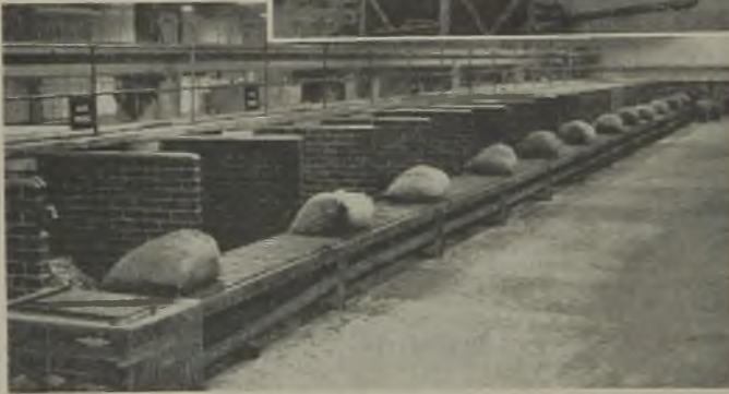
Above: On the first conveyor section the bins pass photo-electric cell equipment (indicated by arrows); guard removed for photograph Left: From the bins the non-ferrous metals are bagged and put on to a slat conveyor
