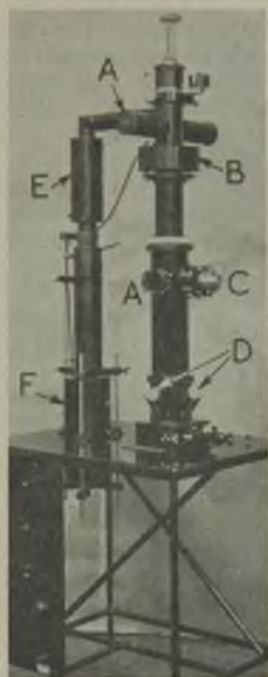
Fig. 8.—Finch-type electron-diffraction camera showing electro-magnetic lens (focusing coil) and vacuum pump A, diaphragms; B, focusing coil; C, specimen port; D, viewing ports; E, mercury vapour trap; F, vapour pump
