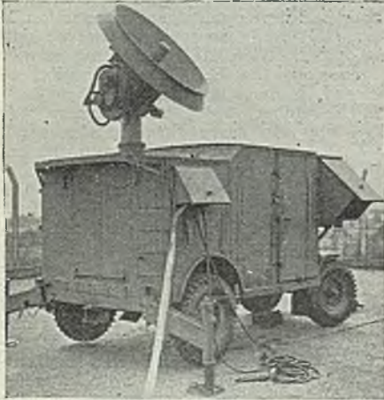
Glaxo, the latest development in A.A. fire control radar, made by the B.T.H. Co.
