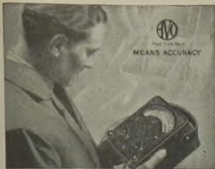
The 50-range Model 7 Universal AvoMeter.
