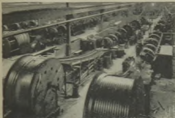
Four armouring machines engaged in reinforcing "Hais" cable with steel tapes and wire armour
