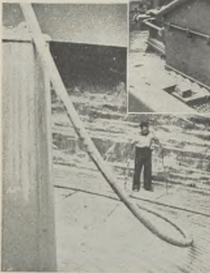
"Hais" cable in the hold of H.M.S. Latimer in one continuous length and (above) cable passing round the cable drum for controlling the speed of laying on board the ship
