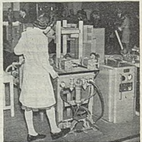
Here 16 glued joints in a desk are drying simultaneously in a jig supplied with power from a R.T.7 2kW unit
