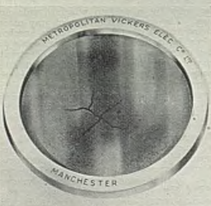
Example of crack detection by residual magnetism, using a captive fluid detector
