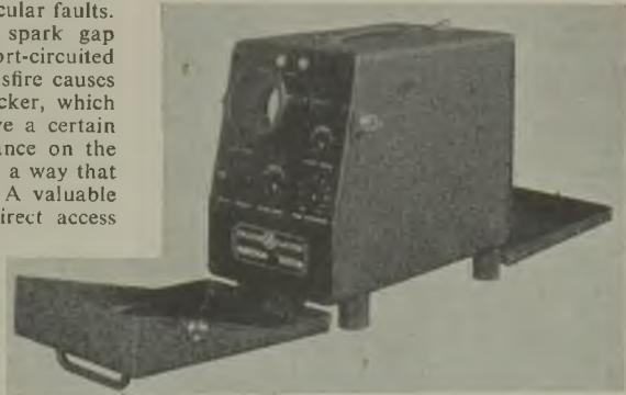
"Tropicalised" cathode-ray ignition tester for the Services
