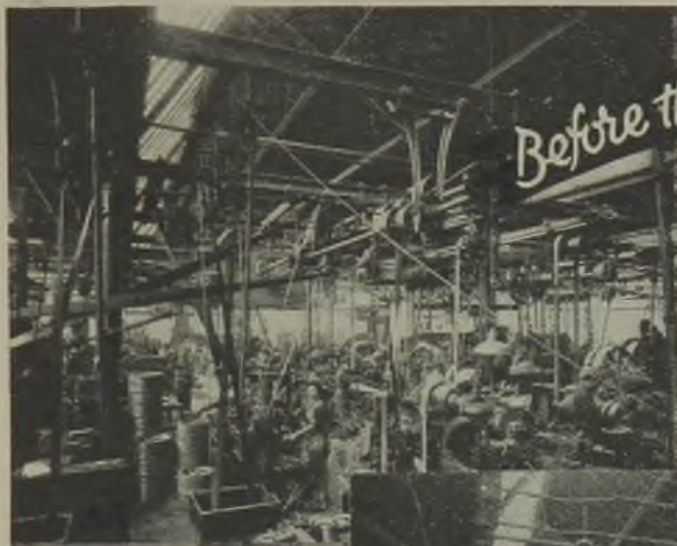
View in a factory containing 105 belt driven machine tools.
