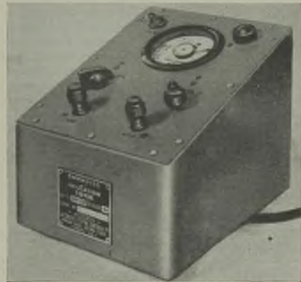
Fig. 2.—Second prototype electronic ohmmeter
