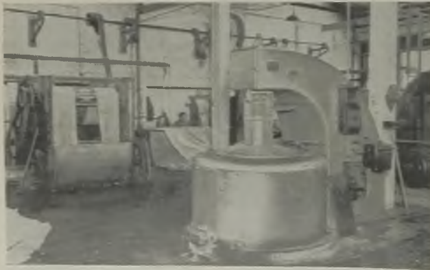
Blanket making at Galston: shrinking machine rear left; centrifugal dryer, right front; picking out knots and loose ends from blanket, rear right
