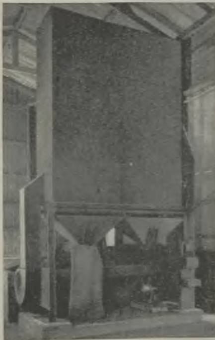
This one-ton-an-hour grain dryer at Rock Moor is driven by a 5-HP motor
