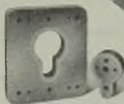
Punch and die after finish grinding
