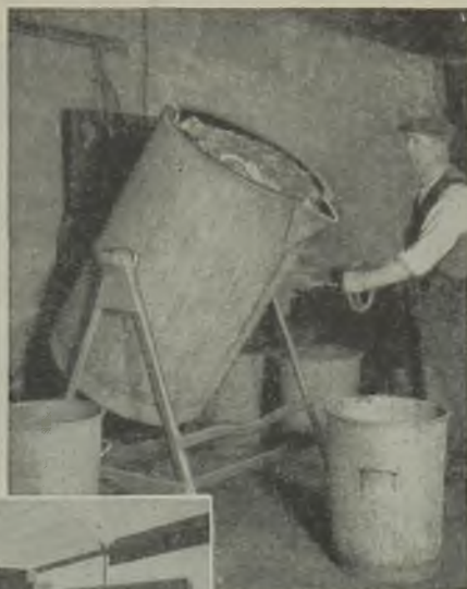
Pig food boiler designed by Nesco staff in use at Rock Farm
